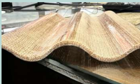
In some cases, less familiar materials were tested, including insulated sandwich panels in Bangkok and experimental jute-resin composite sheets in Dhaka.
