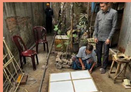
In Dhaka, inexpensive insulation panels were tested as removable layers to reduce heat gain.
