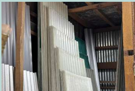
Locally available translucent sheets inspired daylighting solutions in Dhaka, reducing indoor lighting needs.
