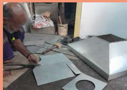
Local artisans then fabricated and tested the kitchen hood, adjusting dimensions and materials.
