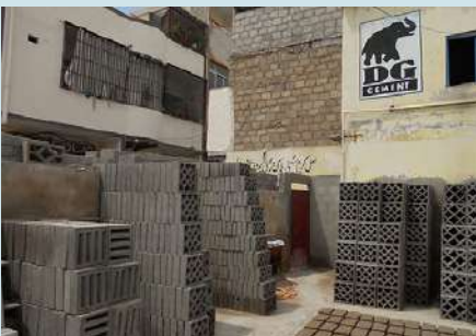
Concrete lattice elements commonly used in Karachi.
